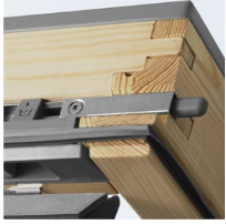
6 Barrel bolt The roof window can be rotated and secured in position with a barrel bolt to ensure safe and easy cleaning of the outside pane from the inside
